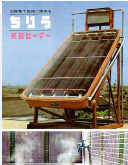
This type of collector was very popular in Japan in the 1960s. The pipes in the case are, at the same time, storage tanks and collectors – made of PVC, PVC clad steel or sometimes FRP (Fibreglass Reinforced Polyester). The disadvantage was the high loss of heat at night and in winter times.
